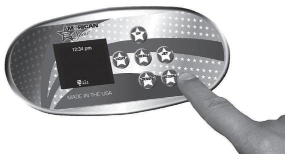
For **NEO 1100**. Press the **RETURN** button on the control panel. After two minutes, the pump should prime. If it does not, follow the priming instructions on the next page. If it does, continue with the next step.
